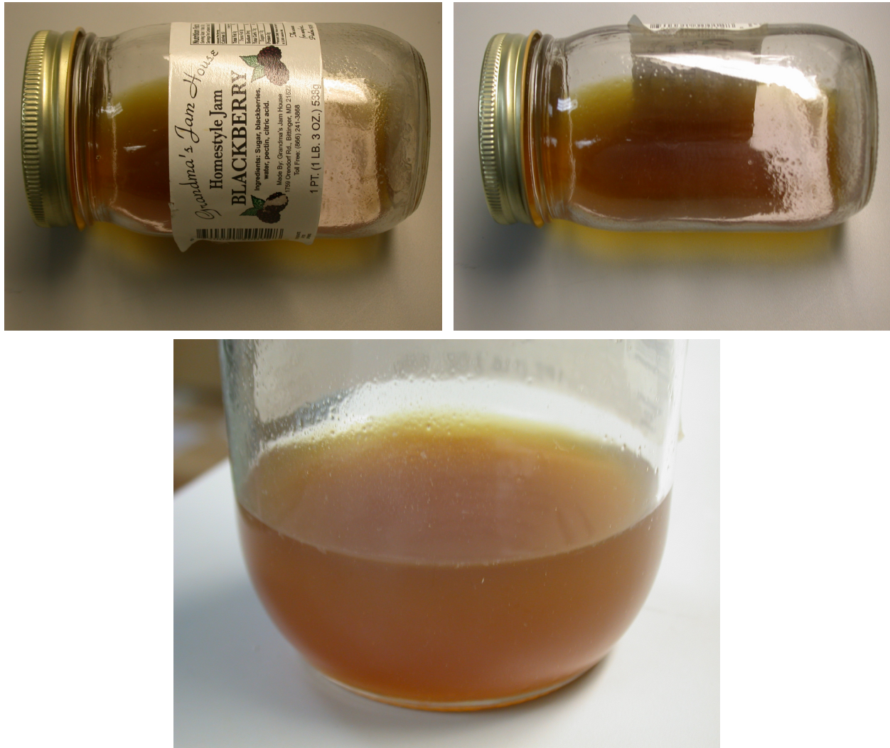
Fig. 1. The liquid for identification and analysis received from the homeowner is shown above as it was received. The jar was well-sealed. Note that the reflection of light from the right side of the liquid surface in the upper right image makes it clear the liquid is more dense than water and has constituents in it which are not uniformly dissolved. The lower image was made soon after returning the jar to its upright position and a thick and rather lumpy residue is seen on the glass surface which has not yet had time to descend into the lower pool of liquid.
