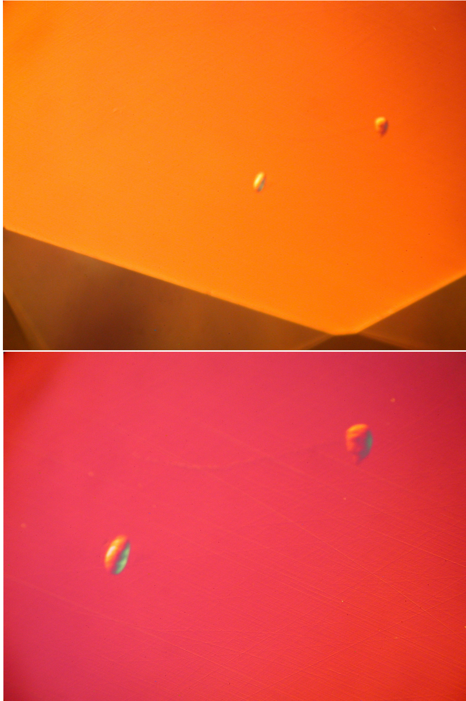
Fig. 6. The front facet of the gemstone as observed by a metallographic microscope. These images were made using Nomarski differential interference phase contrast, which changes the color, but helps to resolve surface features with respect to height differences, chemical differences, and optical index of refraction differences. The two mounds shown here were surface contamination, which moved and changed with each cleaning of the surface. The upper image has a magnification of 185 times, while the lower image is magnified 348 times as-printed.
